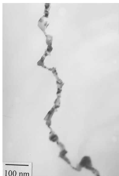
Fig. 2 TEM image of the product obtained by irradiating the solution containing 1% HEC and 1 mmol/l \text{AgNO}_3 for 48 h.
