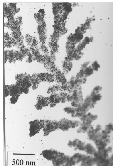
Fig. 3 TEM image of the product obtained by irradiating the solution containing 1% HEC and 50 mmol/l \text{AgNO}_3 .
